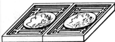
5. Molds show the design in normal position with printing surfaces lower than non-printing ones.
