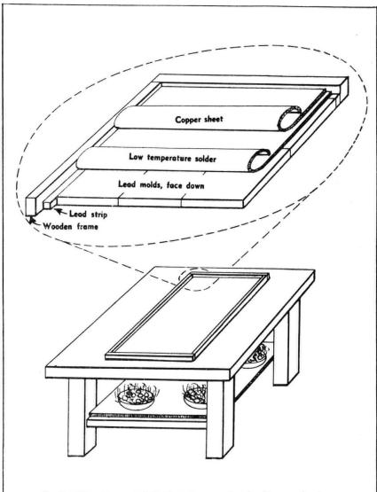
7. The 150 molds are girdled with lead strips and enclosed in a wooden frame. A low-temperature sheet of solder and a thin copper plate cover the assembly. The steel table is heated, melting the solder and fuzing the copper to the lead molds and strips (for electrical conductivity).
