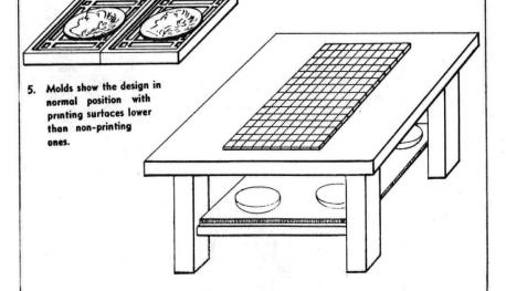
Fifteen rows of 10 molds are laid face down on a steel table to prepare a
