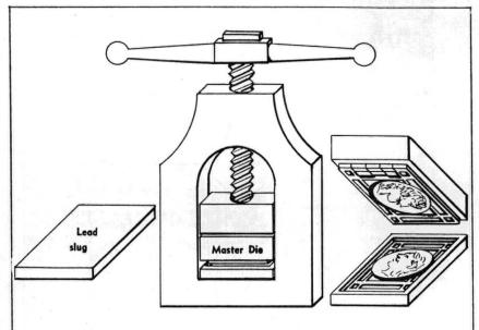
The master die is mounted in a coin press and used to strike lead blocks.
